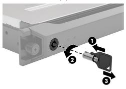
2. Rotate the left side of the bezel off the front of the chassis and then remove the bezel from the chassis.
