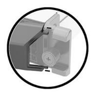
Insert the key into the lock (1), rotate it 90° clockwise (2), and then remove the key (3).
